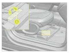
Fold away the floor cover to access the imprinted vehicle identification number (VIN)
