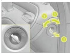
To enable the passenger airbag: pull the switch in the direction of the arrow and rotate the switch counter-clockwise to enable the passenger airbag.
