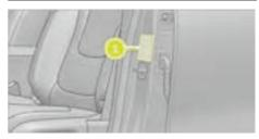
The tyre pressure table is located on the front left B pillar 🕦.
