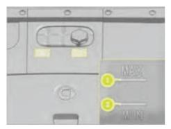
3. If the coolant level is lower than the marked position 1, inspect or top up coolant at a smart Authorized Service Partner
