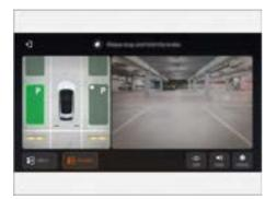
1. When the vehicle speed is below 30 km/h, tap to enter the application interface and tap to enter the Automatic Parking Assist interface, or press the button on the steering wheel to enter the Automatic Parking Assist interface.
