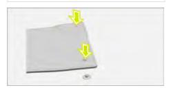
When installing the floor mats, place the floor mats in the correct position, align the floor mat eyelets with the floor mat retaining clips, and then press to lock.
