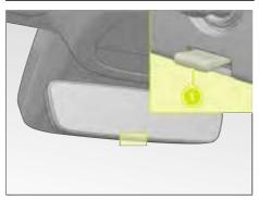
Push the handle at the bottom of the inside rearview mirror to change the view angle to achieve anti-dazzle function. Pull back the handle to return the inside rearview mirror to the normal position and disable the anti-dazzle function.
