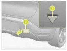
4. Press the lower point of the triangular indicator inward to remove the tow bar cover i.
