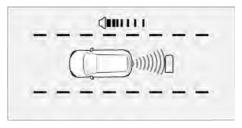
After the vehicle is started, the rear radars are automatically activated when the vehicle is shifted to reverse R and the vehicle speed is below 15 km/h(10 mph). The sound warning signal will be enabled if the vehicle is about 1.5 meters from the rear object.
