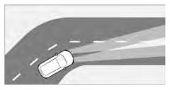
Corner lighting can provide a wide range of lane lighting effect in the turning direction of the vehicle, making it easier to see the road conditions within the turning range.
