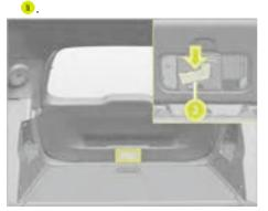
Press the unlock switch and the liftgate unlocks.
