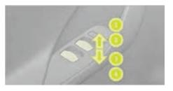
One touch up Pull the button past the point of resistance and release, the window will be closed fully.
