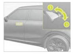
3. Unlock the door: insert the mechanical key into the key hole until it stops, rotate the mechanical key in the direction release the key, release the door
