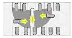
When you are reversing out of your parking space or garage, Rear Cross Traffic Alert alerts you of the vehicle in the rear to avoid collision if there is a risk of a side collision. If necessary, brake will be applied automatically.
