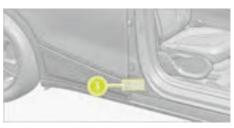
The vehicle identification plate 🕩 is located on the lower section of the right front side B pillar.
