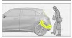
When the vehicle detects the keyfob or smart APP Bluetooth key (if equipped), you can open, close, or stop the liftgate by kicking below the rear bumper.
