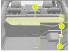
To remove: pull out and remove the boot separator 🕕.
