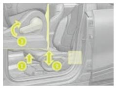
Adjusting the seat forward or backward: lift the lever and slide the seat forward or backward, and lower the lever to engage the seat into position.
