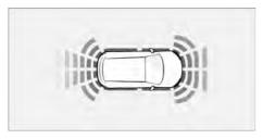
The system uses distance indicator/fan area to indicate objects detected.
