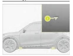
Lifting point indicator • under the door sill outer decoration panel.
