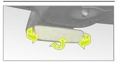
The inside rearview mirror is fixed to the front windscreen and can be turned in the direction of the arrow to the required position.
