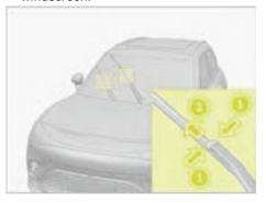
Hold the wiper arm with one hand, press the clip inward along the direction of the arrow 1, and pull the blade out along the direction of the arrow with the other hand.
