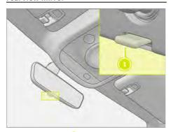
Push the handle 1 at the bottom of the inside rearview mirror to change the view angle to achieve anti-dazzle function. Pull back the handle 1 to return the inside rearview mirror to the normal position and disable the anti-dazzle function.
