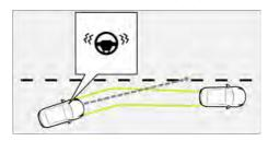
If the driver does not actively control the vehicle and the system detects that the vehicle is deviating from the current lane, the Lane Departure Prevention will actively request steering to help the vehicle return to the current lane. If the vehicle continues to deviate from the lane and is about to cross or crossing the lane line, Lane Departure Prevention will issue a warning if Lane Departure Warning is enabled.
