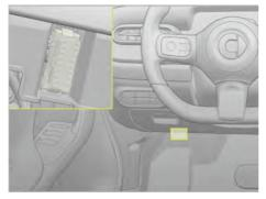
Vehicle identification number (VIN) can be retrieved by a diagnostic scan tool through the diagnostic system interface.
