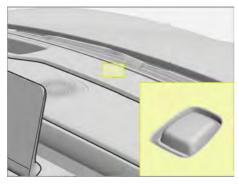
The light sensor is located in the centre of the instrument panel, and the automatic wipers/automatic headlamp/automatic air conditioning control the corresponding functions through this sensor.
