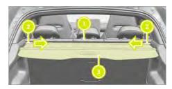
Removal: fold the second row seat backs 1 (→ Page 57), press the boot curtain shaft sleeve 2 toward the centre, and remove the boot curtain 3 forward from the groove.
