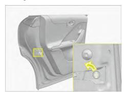
Turn the door lock in the direction of the arrow until it stops. The door will be locked once closed.
