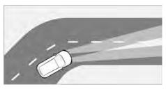
Corner lighting can provide a wide range of lane lighting effect in the turning direction of the vehicle, making it easier to see the road conditions within the turning range.
