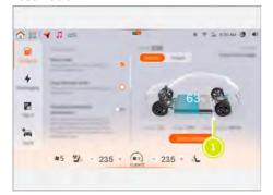
Charging schedule: the user can set the charging schedule on the centre display, and slide the bar leftward or rightward to set the target SOC. Based on the start and end time of charging set by the user and the set target SOC, the vehicle can charge the battery to the target SOC.
