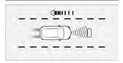
The front radars are enabled automatically when the speed is below about 15 km/h(10 mph) after starting the vehicle. The farthest distance monitored in front of the vehicle is about 1.0m.
