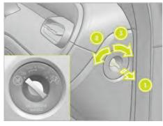
To enable the passenger airbag: pull the switch 1 in the direction of the arrow and rotate the switch counter-clockwise 2 to enable the passenger airbag.
