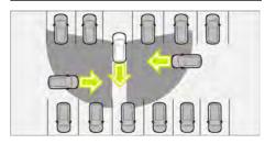
When you are reversing out of your parking space or garage, Rear Cross Traffic Alert alerts you of the vehicle in the rear to avoid collision if there is a risk of a side collision. If necessary, brake will be applied automatically.
