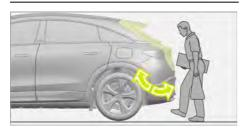
When the vehicle detects the keyfob or smart APP Bluetooth key, you can open, close, or stop the liftgate by kicking below the rear bumper.
