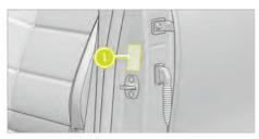
The tyre pressure table is located on the left B pillar 1.
