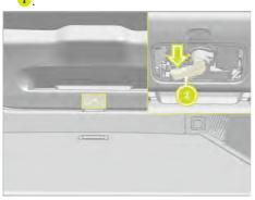
Press the unlock switch 2 and the liftgate unlocks.
