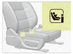
Before every trip, make sure that the ISO-FIX/i-Size child restraint system is engaged correctly in both anchor points on the seat.
