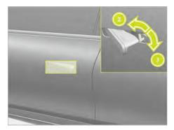
Unlock the door: insert the mechanical key into the key hole until it stops, rotate the mechanical key in the direction
