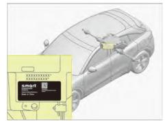
The label indicating the model and serial number of the rear E-motor is situated beneath the back part of the motor.
