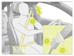
1. Always insert a seat belt tongue 2 into the buckle 1 of the corresponding
