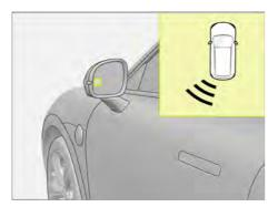
If Door Opening Warning detects the target and a collision risk when the door is open, the system will flash the outside rearview mirror indicator and issue a sound warning, and the driver information display will show the corresponding object warning prompt.
