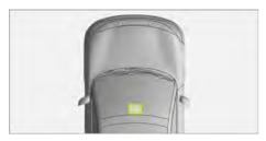
The rain light sensor is located on the upper part of the front windshield, and the automatic wipers/automatic headlamp/automatic air conditioning control the corresponding functions through this sensor.
