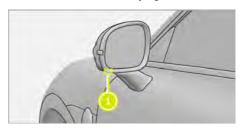
When the vehicle is unlocked, the courtesy light 1 below the outside rearview mirrors automatically illuminate.
