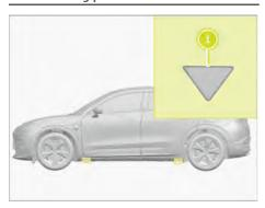
Lifting point indicator 1 under the door sill outer decoration panel.
