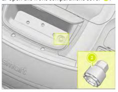
Remove the tool kit, flip open the foam base at the button of the front compartment, and then take out the anti-theft wheel bolt adapter 2 at the location shown in the figure.
