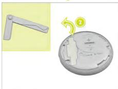
2. Open the mechanical key cover in the direction of the arrow 2 and take out the mechanical kev.
