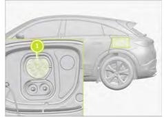
Vehicle discharging port location 1. Vehicle as power source
