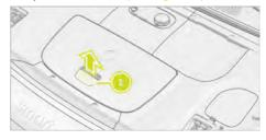
2. Pull the front luggage compartment cover handle 1 upward to open the cover.
