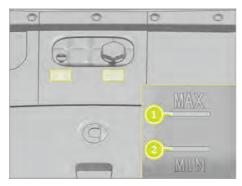
If the coolant level is lower than the marked position <sup>2</sup>, inspect or top up coolant at a smart Authorized Service Partner
